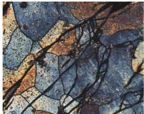
Figure 4: Image showing cracks in etched material passing through grains
